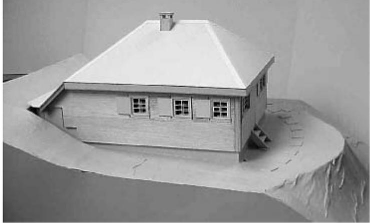
10. Model showing the hut sitting on its leveled shelf of ground, which both cuts into the valley slope and projects from it.
