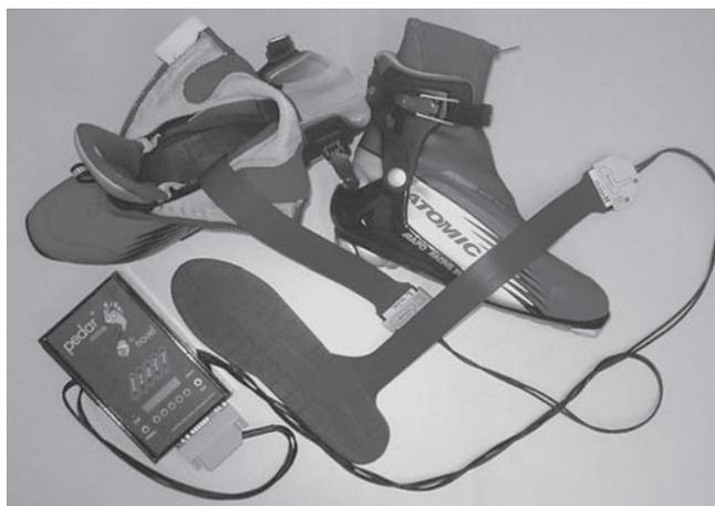
Figure 13.3 Pedar insoles and data storage unit.
