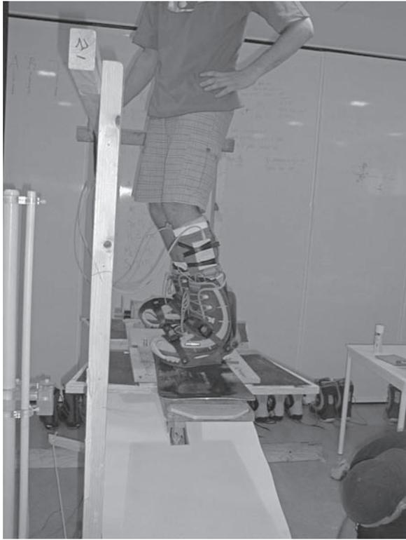
Figure 21.2 The laboratory drop tester; used to simulate snowboard landings at the University of Otago, Department of Physical Education.
