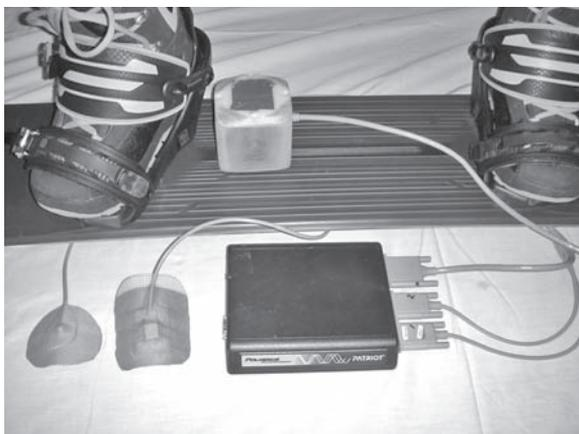
Figure 21.4 The Polhemus Patriot® 3D electromagnetic tracking system. The transmitter mounted to the snowboard with both sensors attached to thermoplastic moulds.
