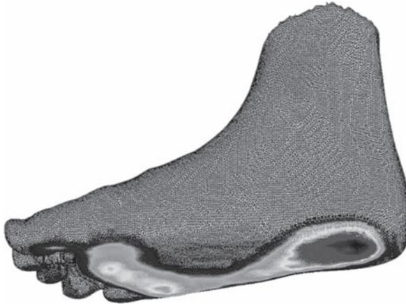
Figure 11.2 Visual combination of foot morphology and pressure distribution data from a 3D laser foot scanning device (LFSD) and a pressure platform.
