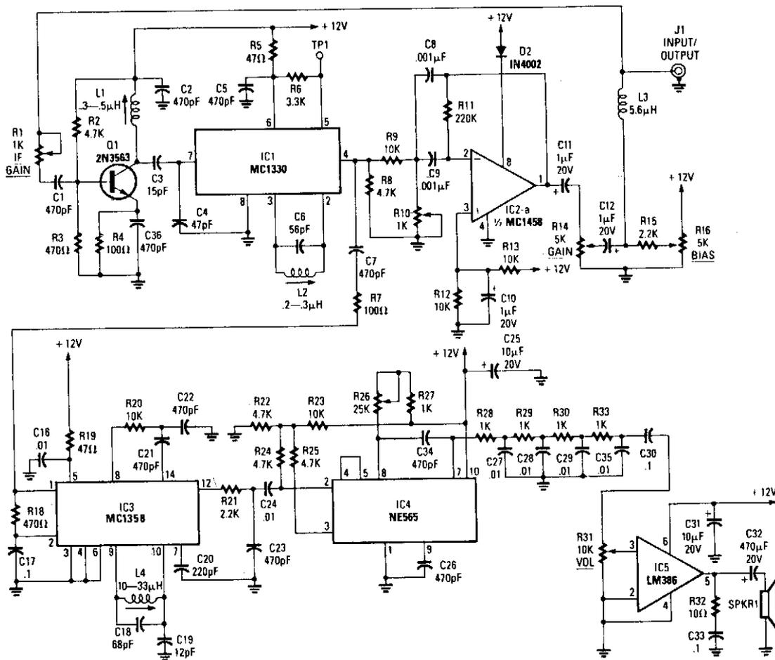
—A COMPLETE SINEWAVE DESCRAMBLER. Easy to build, and relatively easy to align, this circuit completely removes the 15.75-kHz scrambling sine wave.
