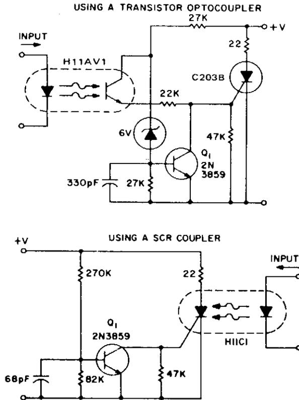
NORMALLY OPEN, TWO TERMINAL, ZERO VOLTAGE SWITCHING HALF WAVE CONTACT CIRCUITS
