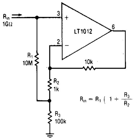
$$R_{in} = R_1 \left( 1 + \frac{R_3}{R_2} \right)$$
