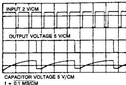
$$R_B = 12500 \text{ } \Omega = .02 \text{ } \mu\text{F}$$
