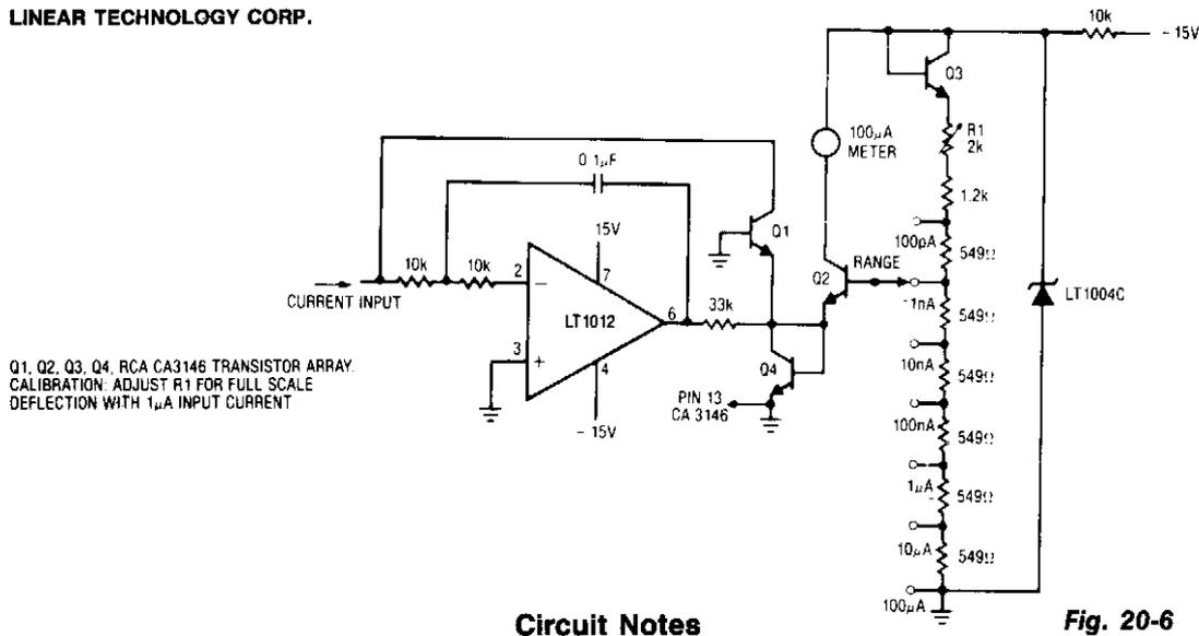
Q1, Q2, Q3, Q4, RCA CA3146 TRANSISTOR ARRAY.
