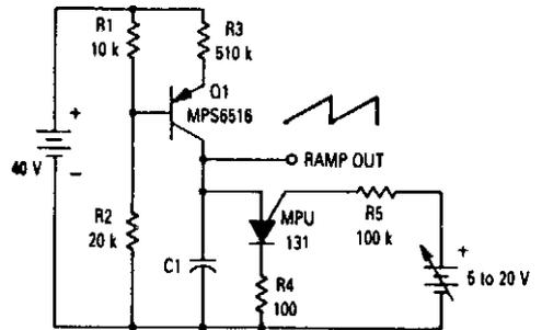
Voltage Controlled Ramp Generator (VCRG)
