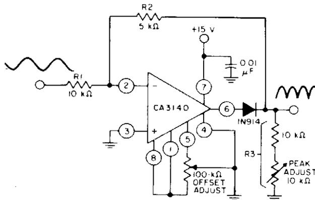
$$\text{GAIN} = \frac{R_2}{R_1} = X = \frac{R_3}{R_1 + R_2 + R_3}$$
