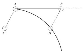
Fig. 2.4 The trajectory of a moving body that has received a blow or has been struck by an impulsive force. There can be no doubt that the force is a thrust, an instaneous force, a force of impact, or a force of percussion, since the text reads that the imparted motion "is proportional to the force."
