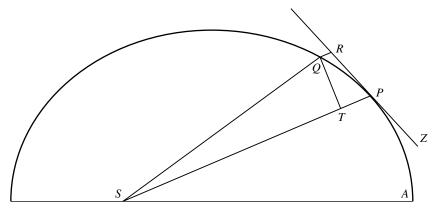
Fig. 3.10 Taken from Proposition 6, Book 1, 1687 *Principia*. The particle at *P* moves along the general curve *APQ* under the influence of a force center at *S*. The line *RPZ* is the tangent to the curve at *P* and the line *QR* is constructed parallel to the line *STP*.
