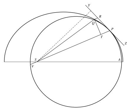
Fig. 3.13 Taken from Proposition 6, Book 1, 1713 *Principia*. In this revised diagram Newton has added the normal to the tangent through the center of force *YS* and has extended the line *SP* to the point *V*, where *PV* is the chord of curvature (the circle of curvature has been added to Newton's diagram).
