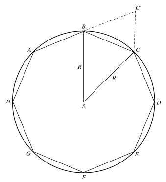
Fig. 3.2 A polygon AB, BC, etc. is inscribed in a circle of radius R. A particle moving with uniform velocity from A to B experiences an impulsive force at B and is then directed toward C. If the impulsive force had not acted, then the particle would have moved to C' in the same time that it moves to C.
