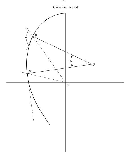
Fig. 3.5 Illustrating how a segment PP' of an orbit is obtained by rotating the radius of curvature vector PQ into P'Q about its fixed center of curvature Q through an angle  $\phi$ , while the center of force is located at C. The dashed lines PC and P'C are the radial positions with respect to C, and the angle alpha is the angle between the tangent to the curve at P and the radial line PC.
