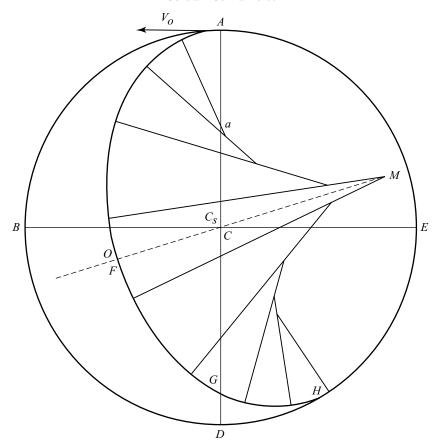
Fig. 3.6 The upper segment AO of the orbit for constant radial force as obtained by the iterations of the curvature method. The point O of closest approach to the center of force C is determined when the curvature vector MO crosses C. Then the lower segment OGH of the orbit is obtained by reflection symmetry of the segment AO about the axis OC.
