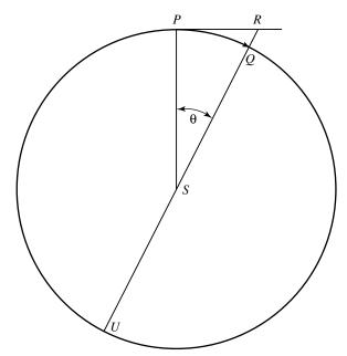
Fig. 3.3 A particle moves along a circular arc from P to Q under the influence of a force directed toward the center of the circle S. The line PR is the tangent to the circle at the point P and the line segment QR is the deviation from the tangent at point Q.
