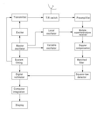
**Figure A92** Block diagram of a radar astronomy system (after Hovanessian, 1984, Fig. 13-5, p. 353).
