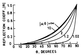
**Figure A11** The angular performance of  $\mu_r = \varepsilon_r$  absorber for different values of  $|\mu\varepsilon|$  (from Bhattacharyya, 1991, Fig. 4.68, p. 215).
