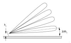
Figure P17 Vertical lobing caused by surface reflec-
