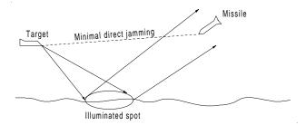
Figure J5 Ground-bounce jamming.
