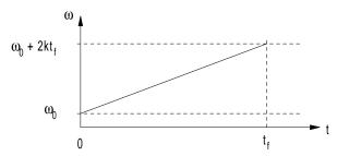
Figure W10 Frequency vs. time for linear FM waveform.
