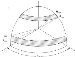
**Figure A46** The solid angle of search, in steradians, for a ground-based radar.
