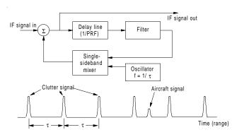
**Figure F26** Coherent memory filter block diagram and output signal (after Skolnik, 1970, Figs. 62, 63, pp. 17.56–17.57).
