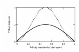
**Figure M29** Velocity response of single- and double-delay MTI cancelers.
