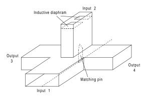
Figure B10 T-type waveguide bridge.
