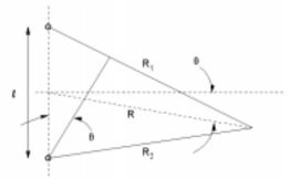
**Figure M18** Geometry of phase-comparison monopulse (after Leonov, 1986, Fig. 1.1, p. 3).
