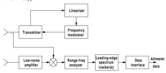
**Figure A23** Block diagram of basic FMCW altimeter (from Cantafio, 1989, Fig. 7.11, p. 247).
