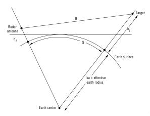
**Figure R86** Ground range *G* in curved-earth reference frame.
