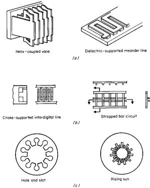
Fig. 9-65. Slow-wave circuits for crossed-field tubes.
