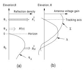
**Figure E11** Multipath reflection density and antenna pattern weighting functions in elevation coordinate. (a) Target and reflection components, (b) sum and difference antenna gains (after Barton, 1988, p. 520).
