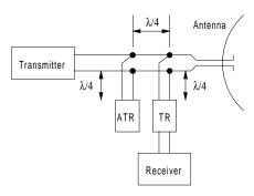
**Figure D59** A branch-type duplexer, parallel configuration (after Skolnik, 1980, Fig. 9.5, p. 360).
