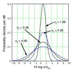
**Figure C25** Log-normal distribution. Median value =  $\sigma_m$ .
