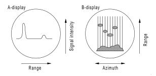
Figure D47 A- and B-displays.
