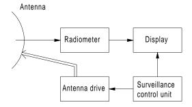
**Figure R50** Scanning thermal-microwave imager (after Nikolaev, 1970, Fig. 28, p. 72).
