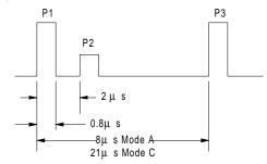
**Figure I11** Interrogation signal format (after Stevens, 1988), Fig. 3.3, p. 23.
