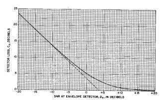
**Figure 18** Envelope detector loss vs. SNR (from Barton, 1988, Fig. 2.2.4, p. 64).
