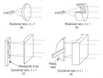
**Figure L2** Basic lens configurations (after Johnson, 1984, Fig. 16.1, p. 16.3).
