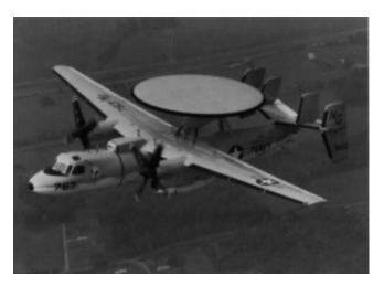
Figure R82 E-2C AEW aircraft with rotodome antenna.
