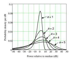
Figure C24 Weibull distribution, plotted as density in dB.
