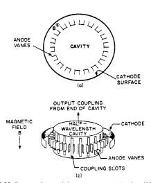
**Figure M3** Inverted coaxial magnetron: (a) simplified cross-section; (b) simplified perspective (from Skolnik, 1990, Fig. 4.5, p. 4.7, reprinted by permission of McGraw-Hill).
