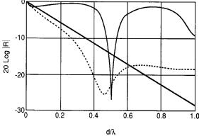
**Figure A4** Reflectivity of dominantly magnetic materials. Solid trace:  $|\mu_r| = 16$ ,  $|\epsilon_r| = 1$ ,  $\delta_\mu = 10^\circ$ ,  $\delta_\epsilon = 0^\circ$ ; dashed trace:  $|\mu_r| = 25$ ,  $|\epsilon_r| = 16$ ,  $\delta_\mu = 20^\circ$ ,  $\delta_\epsilon = 30^\circ$ ; diagonal trace:  $|\epsilon_r| = |\mu_r| = 4$ ,  $\delta_\epsilon = \delta_\mu = 15^\circ$  (from Knott, 1993, Fig. 8.13, p. 319).
