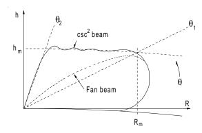
**Figure P5** Example of radar coverage using csc<sup>2</sup> antenna (after Barton, 1988, Fig. 4.2.9, p. 163).
