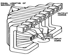
**Figure S9** Organ-pipe scanner (from Brown, in Skolnik, 1970, Fig. 7, p. 22.7, reprinted by permission of McGraw-Hill).
