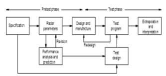
**Figure P8** Flow of radar system design and testing program (after Barton, 1991, Fig. 13.1, p. 13.2).
