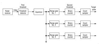
**Figure 15** Block diagram of binary integrator (after Skolnik (1980), Fig. 10.7, p. 388).
