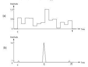
**Figure C34** Matched-filter response to 14-element Huffman code: (a) transmitted amplitude; (b) matched-filter output (after Cook, in Brookner, 1977, p. 146).
