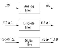
Figure F21 Types of signal-processing filters.
