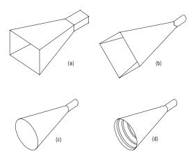
**Figure A59** Common types of horn antennas: (a) pyramidal horn; (b) diagonal horn; (c) conical horn; (d) corrugated horn (after Currie, 1987, Fig. 12.12, p. 539).
