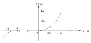
Figure D39 Typical voltage-current response for a PN diode.
