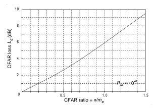
**Figure L23** Universal curve for CFAR loss in single-hit detection, for steady or Rayleigh target (after Gregers-Hansen).
