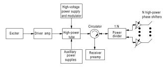
Figure T22 A simplified block-diagram of tube transmitter for phased-array radar (after Ostroff, et al, 1985, Fig. 8.3a, p. 208).
