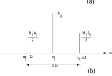
**Figure M12** Amplitude modulation of the signal: (a) amplitude-modulated waveform (the dashed line indicates the envelope); (b) spectrum of resulting signal.
