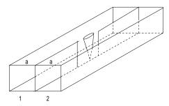
Figure B8 Slotted-waveguide bridge.
