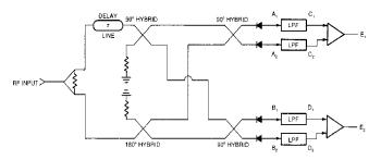
**Figure R94** A typical basic IFM receiver (from Vaccaro, 1993, Fig. 6.1, p. 128).
