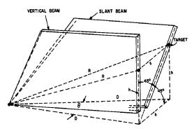
**Figure H3** V-beam geometry (from Fink, 1989, p. 25.49, reprinted by permission of McGraw-Hill).
