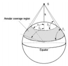
Figure C52 Typical spaced-based radar coverage.
