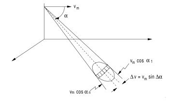
Figure D56 Doppler-beam-sharpening geometry, airborne radar.
