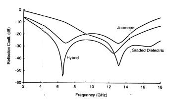
**Figure A8** Reflection coefficient as a function of frequency for Jaumann, graded dielectric, and hybrid absorbers (from Knott, 1993, Fig. 8.28, p. 342).
