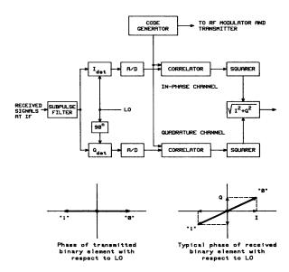
**Figure P25** Digital pulse compression for binary-coded waveform (from Skolnik, 1990, Fig. 10.12, p. 10.23, reprinted by permission of McGraw-Hill).
