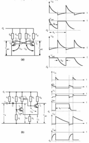
**Figure M33** Multivibrators: (a) in self-oscillating mode, (b) in triggered mode.
