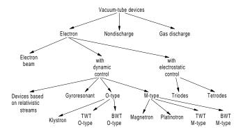
Figure D36 Classification of vacuum-tube devices.
