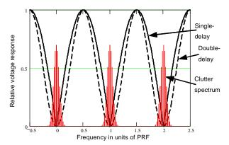
**Figure C1** Relative frequency response of the single-delay canceler (solid curve) and the double-delay canceler (dashed curve). (after Skolnik, 1980).
