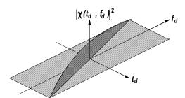
**Figure A33** Knife-edge ambiguity function (after Skolnik, 1980, Fig. 11.13, p. 419).
