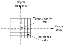
**Figure C36** Use of reference cells from combined range and doppler regions surrounding the target cell.
