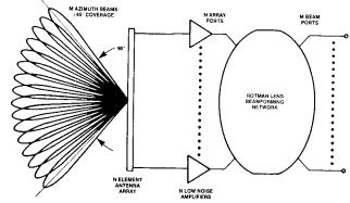
**Figure A88** Rotman lens-fed array for one coordinate (from Barton, 1988, Fig. 4.3.7, p. 178).
