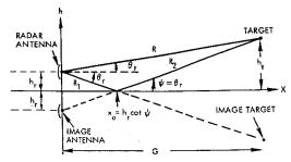
**Figure P18** Multipath geometry over flat Earth.
