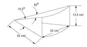
Figure C51 Airborne radar ground coverage.
