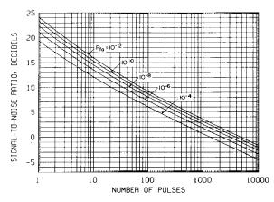
**Figure D15** Detectability factor for  $P_d = 0.9$  using *n*-pulse integration on case 1 fluctuating target (from Blake, 1980, Fig. 2-12, p. 50).
