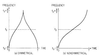
**Figure W13** Nonlinear FM waveforms (from Skolnik, 1990, Fig. 10.2, p. 10.6, reprinted by permission of McGraw-Hill).
