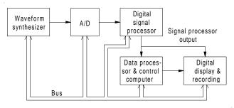
**Figure T14** Signal-processor test configuration (after Barton, 1991, Fig. 13.5.5, p. 13.13).
