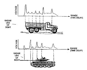
**Figure T6** Ultra-high-resolution profiles of stationary targets (from Currie, 1987, Fig. 6.32, p. 273).
