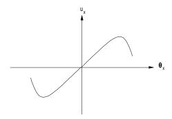
Figure R117 Discriminator response of monopulse system.
