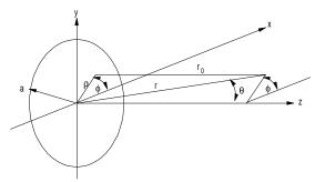
**Figure A52** Planar circular antenna and coordinate system (from Bogush, 1989, Fig. 3.31, p. 146).
