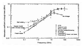
Figure A98 Measured and calculated attenuation coefficient for trees vs. frequency (from Currie, 1992, Fig. 2.19, p. 81).
