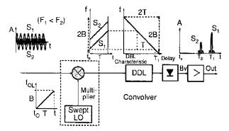
**Figure R99** Microscan receiver (from Neri, 1991, Fig. 4.19, p. 301).
