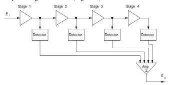
**Figure D31** Basic configuration of a logarithmic detector (after Skolnik, 1970, Fig. 29a, p. 5.34).
