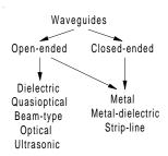
Figure W17 Basic types of waveguide.
