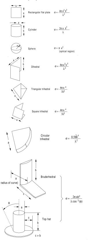
**Figure T1** Characteristics of several typical reference reflectors (after Currie, 1989, Fig. 4.10, p. 107).
