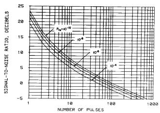
**Figure D16** Detectability factor for  $P_d = 0.9$  using *n*-pulse detection on case 2 fluctuating target (from Blake, 1980, Fig. 2-17, p. 53).
