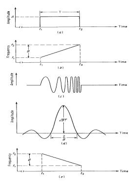
**Figure W11** Linear FM waveform and its compression: (a) transmitted waveform; (b) frequency of the transmitted waveform; (c) representation of the time waveform; (d) output of the pulse-compression filter; and (e) same as (b) but with decreasing frequency (from Skolnik, 1980, Fig. 11.15, p. 423, reprinted by permission of McGraw-Hill).
