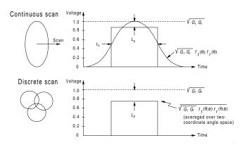
**Figure L19** Definition of beamshape loss for one-coordinate continuous scan and discrete-position raster scan.
