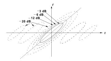
Figure A27 Ambiguity function of an LFM rectangular pulse.
