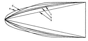
**Figure R85** Five radome shapes, each having a fineness ratio of 2.5. (a) Cone, (b) Von Karman, (c) tangent ogive, (d) Haack, (e) 60° log spiral (from Currie, 1987, Fig. 12.1, p. 569).
