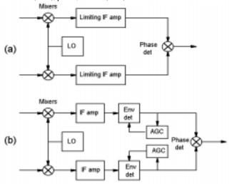
**Figure M20** Phase angle discriminator: (a) with limiting IF amplifiers; (b) with AGC (after Leonov, 1986, Fig. 1.4, p. 10).
