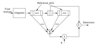
Figure C35 Cell-averaging CFAR (after Skolnik, 1990, Fig. 8.12, p. 8.13).
