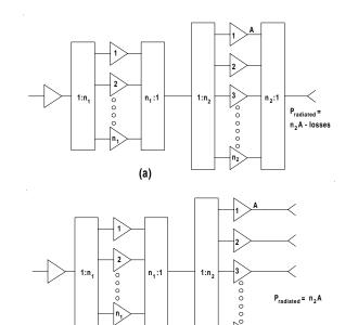
**Figure T21** Block diagram of (a) a corporate-combined power amplifier; (b) a space-combined power amplifier (after Skolnik, 1990, Fig. 5.6, p. 5.12).
