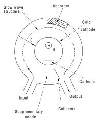
Figure A36 Annular magnetron amplifier.
