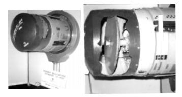
Figure A51 Inverse Cassegrainian antenna: the Cyrano airborne radar.
