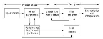
**Figure T12** Flow of radar system design and testing program (after Barton, 1991, Fig. 13.1, p. 13.2).
