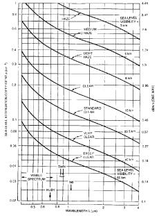
**Figure A100** Approximate variation of attenuation coefficients with laser wavelength, at sea level for various atmospheric conditions, excluding  $\rm H_2O$  and  $\rm CO_2$  components (from Jelalian, 1992, Fig. 2.3, p. 65).
