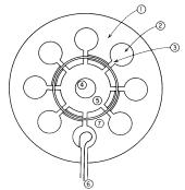
**Figure M2** Cross-sectional sketch of classical cavity magnetron (from Skolnik, 1980, Fig. 6.1, p. 193, reprinted by permission of McGraw-Hill).
