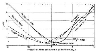
**Figure L25** Filter matching loss vs. filter noise bandwidth  $B_{nh}$  for rectangular pulse of with  $\tau$  with different filters (from Barton, 1969, Fig. 3.17, p. 84).
