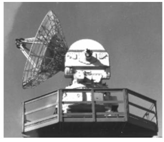
Figure R33 AN/FPS-16 instrumentation radar (RCA photo).
