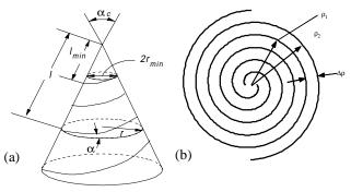
**Figure A67** Log-spiral antennas: (a) conical spiral; (b) planar spiral.
