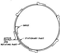
**Figure S13** Ring-switch scanner (from Johnson, 1984, Fig. 18.30, p. 18.25, reprinted by permission of McGraw-Hill).
