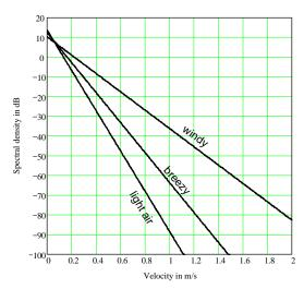
Figure C27 Spectra of windblown tree clutter.
