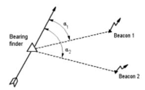
Figure N1 Angle-finding navigation method.
