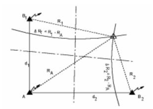
Figure N3 Range-difference navigation method.
