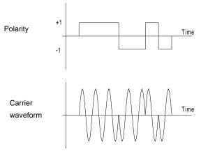
**Figure W6** Binary-coded waveform (after Skolnik, 1990, Fig. 10.8, p. 10.17).
