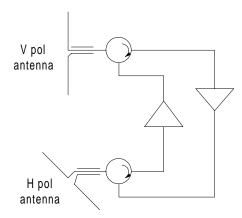
Figure E4 Block diagram of cross-pol ECM.
