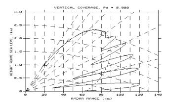
ODERN RADAR SYSTEM ANALYSIS, VERSION 2.03, (C) ARTECH HOUSE 199-Figure C49 2D search radar coverage (from Barton, 1993,
