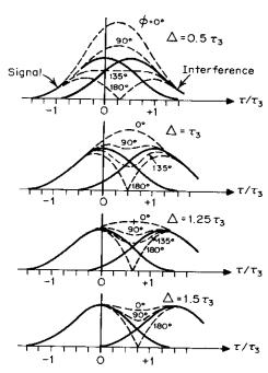
**Figure R113** Resolution between adjacent targets with separations  $\Delta$  and RF phase difference  $\phi$  (from Barton, in Fink, 1982, Fig. 25-28, p. 25-23).
