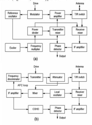
**Figure R14** Coherent pulse radar: (a) coherent; (b) pseudocoherent.
