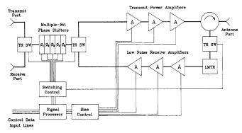
**Figure T18** Block-diagram of transceiver module for phased array (from Skolnik, 1990, Fig. 5.9, p. 5.17, reprinted by permission of McGraw-Hill).
