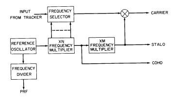
**Figure L11** Local oscillator in frequency multiplication circuit (from Skolnik, 1970, Fig. 11, p. 5-15, reprinted by permission of McGraw-Hill).
