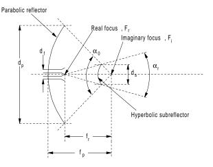
**Figure A50** Cassegrainian reflector antenna. (after Leonov, 1986, Fig. 2.3, p. 15).
