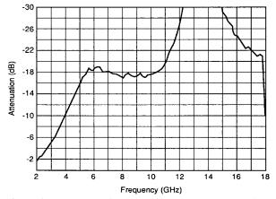
**Figure A7** Measured reflectivity of a three-layer graded dielectric absorber (from Knott, 1993, Fig. 8.17, p. 325).
