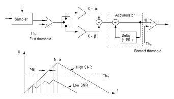
**Figure D6** Accumulator detection (after Neri, 1991, Fig. 2.55,
