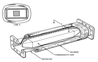
**Figure P11** Typical Reggia-Spencer phase-shifter configuration (from Skolnik, 1970, Fig. 27, p. 12.27, reprinted by permission of McGraw-Hill).
