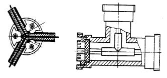
**Figure T7** Coaxial tee configurations: (a) (after Lavrov, 1974, Fig. 18.43, p. 348.
