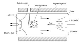
Figure B2 O-type backward-wave tube.
