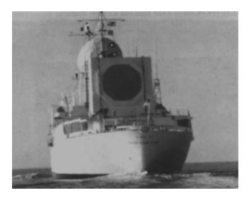
**Figure R62** Cobra Judy reentry observation radar (Raytheon photo).
