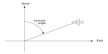
Figure A41 Azimuth angle, measured from north.
