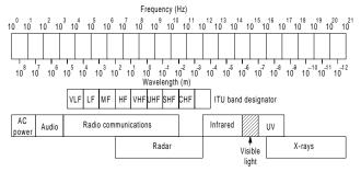
Figure W2 The electromagnetic spectrum.
