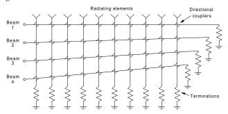
Figure F2 Blass multiple-beam-forming matrix.
