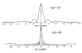
**Figure S23** Linear FM matched-filter response for  $\tau \Delta f = 10$  and  $\tau \Delta f = 50$ ,  $\Delta f$  normalized to unity (from Barton, 1991, Fig. 7.2.4, p. 7.6).
