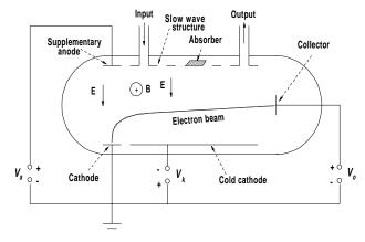
Figure A35 Linear magnetron amplifier.
