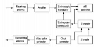
Figure R32 Impulse radar with ultrawideband signal.
