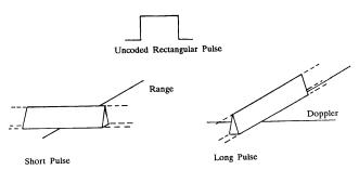
Figure P23 Simple rectangular pulse (from Bogush, 1989, Fig. 3.54, p. 193).
