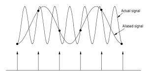
**Figure A20** Aliasing in the time domain (after Currie, 1989, Fig. 6.6, p. 183).
