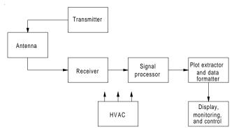
FigureS29 Block diagram of typical radar by subsystems.
