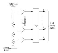
Figure C41 Simultaneous analog-to-digital converter.
