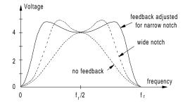
**Figure C2** Frequency response of a double-delay canceler with and without feedback (after Barton, 1964, p. 220).
