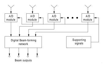
Figure A78 Block diagram of a digital array antenna.
