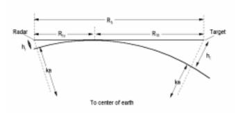
Figure H4 Radar horizon.
