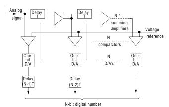
Figure C42 Sequential analog-to-digital converter.
