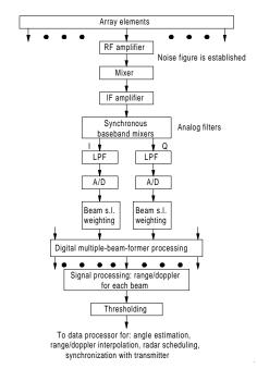
**Figure F6** Digital beam-forming system (after Barton, 1988, Fig. 4.3.12, p. 184).
