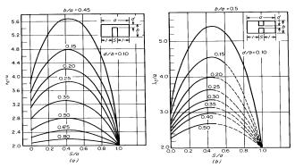
**Figure W22** Cutoff wavelength of ridge waveguide: (a) single ridge; (b) double ridge (from Fink, 1982, Fig. 9-8, p. 9-13, reprinted by permission of McGraw-Hill).
