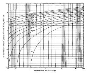
**Figure D13** Detectability factor for single-pulse detection on steady signal (from Blake, 1980, Fig. 2-3, p. 39).
