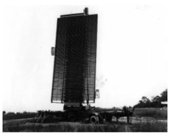
**Figure R64** AN/TPS-59 scanning-beam 3D radar. In this design, each row of elements has its own RF module, containing a power amplifier, a low-noise receiving amplifier, and a phase shifter (General Electric Co. photograph).
