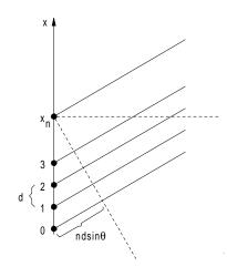
Figure P4 Array elements and coordinates.
