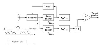
**Figure A17** Automatic acquisition circuit (after Neri, 1991, Fig. 2.72, p. 148).
