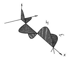
Figure W1 A plane electromagnetic wave.
