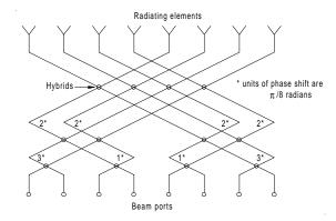
Figure F3 Butler multiple-beam-forming matrix.
