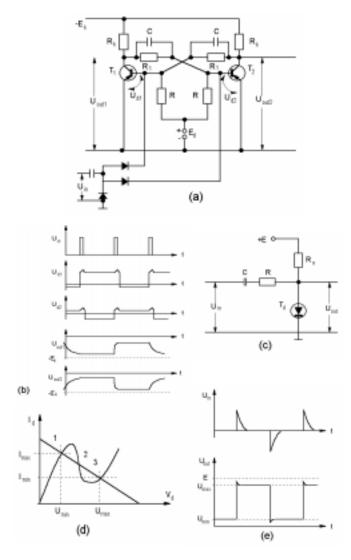
**Figure T28** Flip-flops: (a) symmetrical, (b) voltages of symmetrical flip-flop, (c) tunnel diode type, (d) characteristic of a tunnel diode, (e) voltages of tunnel-diode flip-flop (after Druzhinin, 1967, Fig. 6.26, page 240 and Fig. 6.30, page 243).
