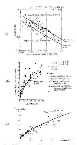
**Figure A101** Attenuation coefficients for laser propagation (a) in fog; (b) in rain; (c) in snow (from Jelalian, 1992, pp. 72–74).
