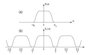
**Figure 2** Spectra before and after sampling: (a) analog signal spectrum, (b) discrete waveform spectrum for  $T = \pi/\omega_m$ .
