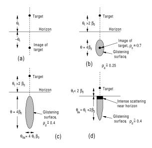
**Figure E10** Multipath reflections for (a) smooth surface, (b) slightly rough surface, (c) rough surface, and (d) rough surface with low-elevation target (after Barton, 1969, p. 150).
