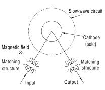
**Figure C55** Simplified representation of circular-format CFA (after Ewell, 1981, Fig. 2-12, p. 38).
