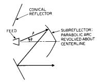
**Figure 104** Conical reflector antenna (from Johnson, 1993, Fig. 17.13, p. 17.13).
