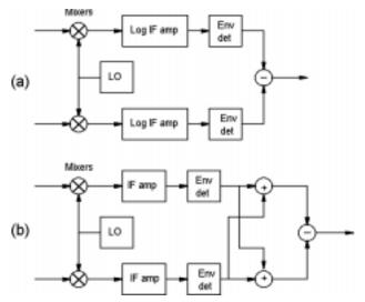
**Figure M19** Amplitude angle discriminator: (a) with logarithmic IF amplifiers; (b) with normalization of the sum at video frequency (after Leonov, 1986, Fig. 1.3, p. 9).
