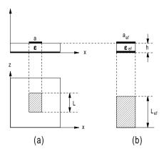
**Figure R116** Resonators: (a) based on asymmetrical microstrip line; and (b) Oliner model (after Veselov, 1988, Fig. 2.17, p. 48).
