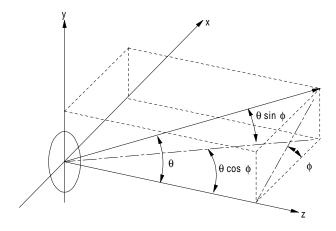
Figure C45 Spherical coordinate system.
