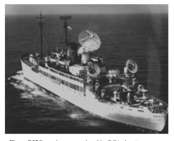
Figure R35 Range instrumentation ship (RCA photo).
