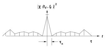
Figure A28 Ambiguity function of a PSK pulse.
