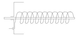
**Figure A58** Helix antenna (after Macnamara, 1995, Fig. 5.18, p. 161).
