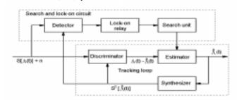
**Figure F34** Tracking loop filter diagram (after Korostelev, 1987, Fig. 8.4, p. 267).
