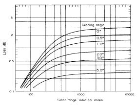
Figure L18 Atmospheric lens loss (two-way) vs. range, for different elevation angles (after Weil).
