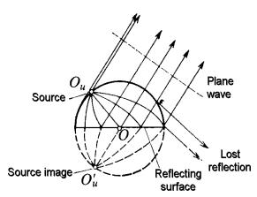
**Figure L5** Hemispheric Luneburg lens (from Leonov, 1986, Fig. 2.8, p. 20).
