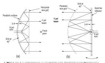
(a) Folded parabolic geometry, (b) mirror-scan geometry.
