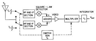
**Figure R80** Parallel-channel (Graham's) receiver (from Skolnik, 1970, Fig. 17, p. 39.17, reprinted by permission of McGraw-Hill).
