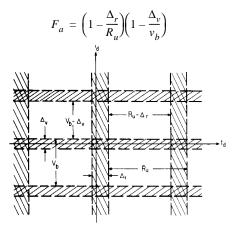
**Figure P30** Blind regions in MPRF PD radar (from Barton, 1988).
