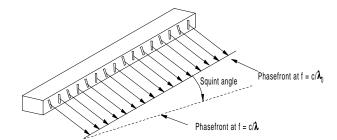
Figure A48 Squint angle in radiation from slotted waveguide.
