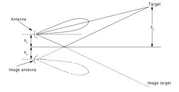
Figure A62 Geometry of the "image" antenna.
