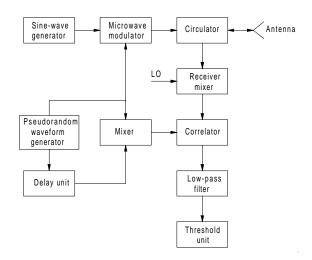
Figure R47 Radar with pseudonoise waveform.
