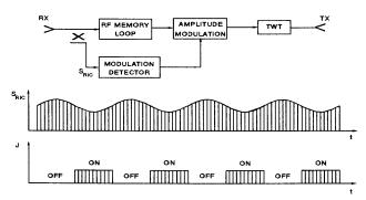
**Figure G1** Inverse-gain jamming waveform (from Neri, 1991, Fig. 5.33, p. 381).
