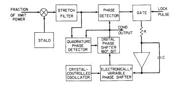
**Figure L13** Phase-shift COHO (from Skolnik, 1970, Fig. 14, p. 5-17, reprinted by permission of McGraw-Hill).
