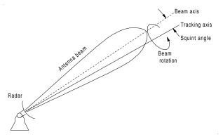
Figure A47 Squint angle in conical scanning.
