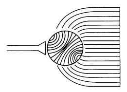
**Figure S10** Organ-pipe (rotary) scanner (from Johnson, 1984, Fig. 18.27, p. 18.24, reprinted by permission of McGraw-Hill).
