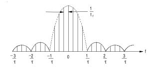
Figure P22 Spectrum of coherent pulse train.
