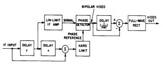
**Figure M32** Phase-detection circuit for noncoherent MTI (from Skolnik, 1970, Fig. 59, p. 17.54, reprinted by permission of McGraw-Hill).
