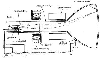
**Figure C12** Cathode-ray tube (from Fink, 1982, p. 11.49, reprinted by permission of McGraw-Hill).
