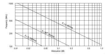
**Figure A99** Ionospheric attenuation as a function of frequency, one-way transmission path (after Berkowitz, 1965, Fig. 1.32, p. 376).
