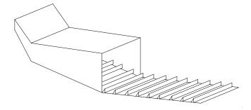
Figure A63 Impedance antenna.
