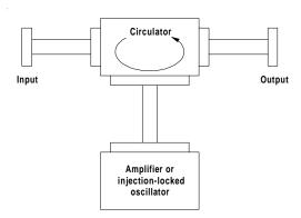
**Figure A38** Single-port amplifier (after Currie, 1987, Fig. 8.8, p. 406).
