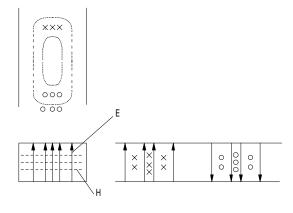
**Figure W21** Structure of field of H<sub>10</sub> wave in rectangular waveguide (after Nikol'skiy, 1964, Fig. 210, p. 275).
