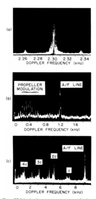
**Figure T5** Pulse-doppler spectrum measurements showing (a) an AM sideband pair caused by a conical-scan radar antenna; (b) FM modulation from propellers of a DC-7 aircraft; and (c) jet engine modulation at the compressor rotation rate and its harmonics (from Skolnik, 1970, Fig. 17, p. 28.22).
