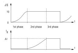
Figure E5 Range gate pull-off operation.
