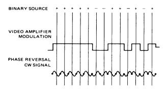
**Figure W5** Waveforms for a Barker code of length 13 (from Hovanessian, 1984, Fig. 8-24, p. 241).
