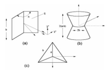
**Figure R105** Corner reflectors: (a) dihedral, (b) biconical, (c) trihedral.
