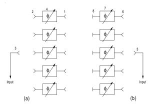
**Figure F16** Space-fed arrays: (a) transmission feeds; (b) reflection feeds.
