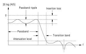
Figure F23 Deviations of characteristic of real filter from ideal characteristics (from Siebert, 1986).
