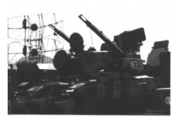
$\label{eq:Figure R21} \textbf{Russian antiaircraft gun and missile system, using S-band search and $K_u$-band fire control radar.}$
