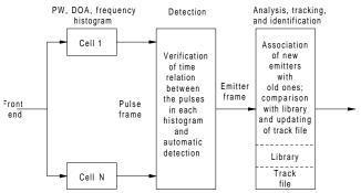
**Figure D26** Open-loop automatic detection (from Neri, 1991, Fig. 4.27, p. 310).
