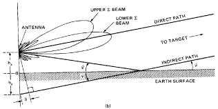
**Figure H2** Multipath effects on monopulse and squinted-beam height finders: (a) conventional  $\Sigma$ , $\Delta$  monopulse, (b) squinted-beam low-angle technique (from Skolnik, 1990, Fig. 20.12, p. 20.37, reprinted by permission of McGraw-Hill).
