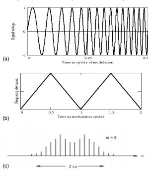
**Figure M13** Frequency modulation of the signal: (a) FM waveform; (b) frequency vs. time; (c) FM spectrum.
