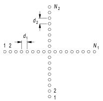
Figure A84 Mill's cross antenna array.
