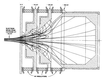
**Figure T25** Multiple depressed collectors in TWT (from Skolnik, 1990, Fig. 4.11, p. 4.18, reprinted by permission of McGraw-Hill).
