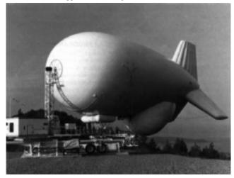
**Figure R1** Small aerostat surveillance system, designed by Westinghouse for battle field surveillance, using a modified AN/APG-66 AI radar.
