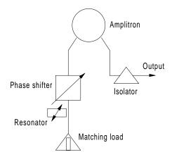
Figure S26 Stabilitron circuit (after Dulin, 1972, Fig. 6-19, p. 130).
