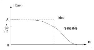
Figure F32 Low-pass filter frequency response.
