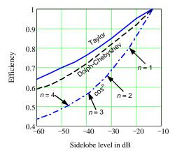
**Figure L24** Doppler filter weighting efficiency vs. sidelobe level for different families of weighting function.
