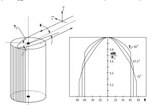
Figure R106 Cylindrical Luneburg reflector and its scattering pattern.
