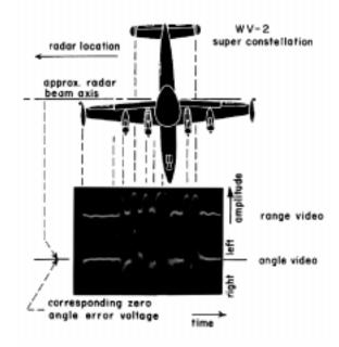
**Figure R31** High-range-resolution monopulse range and angle video from a Super-Constellation aircraft in flight (from Skolnik, 1990, Fig. 18.28, p. 18.32, reprinted by permission of McGraw-Hill).
