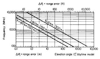
**Figure E19** Ionospheric range error vs. frequency (from Barton, 1988, p. 312).
