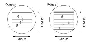
Figure D48 C- and D-displays.
