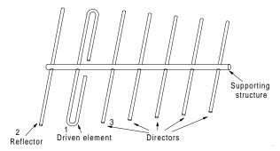
Figure A91 Yagi-Uda array.
