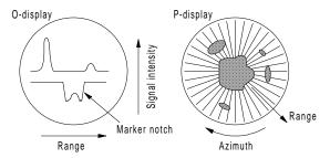
Figure D54 O- and P-displays.
