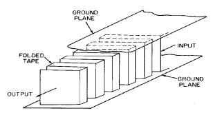
**Figure D2** Tapered folded-tape meander line (from Skolnik, 1970, Fig. 10, p. 20.12, reprinted by permission of McGraw-Hill).
