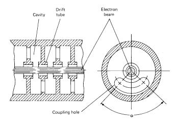
**Figure T24** Coupled-cavity approach for slow-wave circuit in a TWT (from Ewell, 1981, Fig. 2.35c, p. 65).
