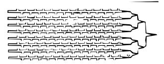
**Figure A83** Photo mask for a microstrip array antenna (from Leonov, 1988, Fig. 5.4, p. 168).
