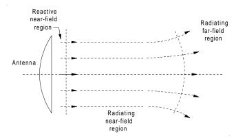
**Figure A72** Electromagnetic field regions in front of antenna (after Johnson, 1993, Fig. 1-7, p. 1.11).
