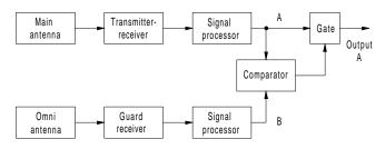
**Figure B5** Sidelobe blanker in which the output A is inhibited if signal B exceeds A (after Long, 1992, Fig. 6.13, p. 248).
