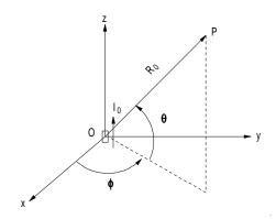
Figure F20 Geometry of the antenna field.
