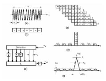
Figure P28 Compression of a phase-coded signal.
