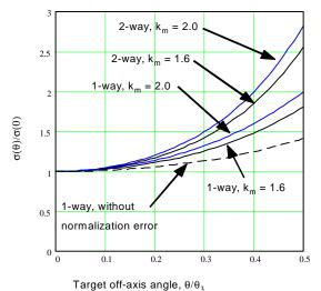
**Figure A13** Ratio of monopulse off-axis error to on-axis error (from Barton, 1969, Fig. 2.12, p. 43).
