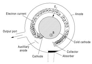
Figure B1 M-type backward-wave tube.
