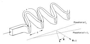
**Figure F14** Serpentine feed for frequency-scanning radar (from Barton, 1988, Fig. 4.3.2, p. 169).
