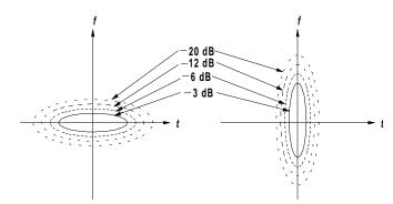
Figure A24 Two-dimensional ambiguity diagram of a single Gaussian pulse. (a) long pulse; (b) short pulse. The contours indicate levels relative to the central response.
