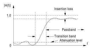
Figure F29 High-pass filter response.
