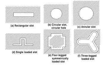
**Figure A5** Frequency-selective surfaces (after Knott, 1993, Fig. 8.22, p. 330).
