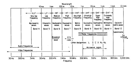
**Figure F38** Radar portion of the electromagnetic spectrum (from Skolnik, 1980, Fig. 1.4, p. 7, reprinted by permission of McGraw-Hill).
