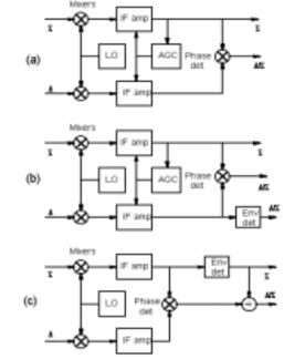
**Figure M21** Sum-and-difference angle discriminators: with (a) combined, and (b) separate formation of the magnitude and sign of the error signal, and (c) with normalization by the sum signal at video frequency (after Leonov, 1986, Fig. 1.5, p. 11).
