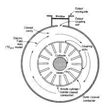
**Figure M1** Cross-sectional sketch of the coaxial cavity magnetron (from Skolnik, 1980, Fig. 6.3, p. 194, reprinted by permission of McGraw-Hill).
