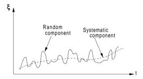
Figure E8 Radar measurement error.
