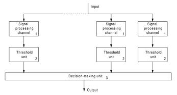
Figure D24 Multichannel detector.
