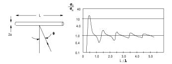
Figure R107 Dipole reflector and its RCS variation with length.
