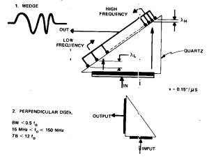
**Figure D1** Diffraction-grating delay line (from Brookner, 1970, Fig. 30, p. 138).
