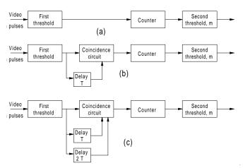
**Figure D12** Principle of coincidence detection: (a) no coincidence; (b) double coincidence; (c) triple coincidence (after DiFranco, 1980, Fig. 14.5-1, p. 515).
