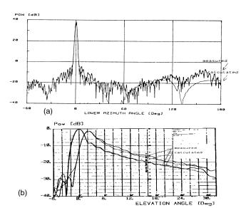
**Figure P1** Example of search radar antenna patterns in principal planes: (a) azimuth pattern; (b) elevation pattern.
