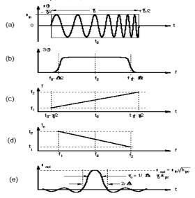
**Figure P27** Compression of a linear-FM (chirp) signal (after Fal'kovich, 1989, Fig. 6.13 and 6.14, page 245).
