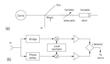
**Figure B7** The Marsh and Wiltshire bridge: (a) bridge circuit, (b) noise cancellation circuit using the bridge (after Skolnik, 1990, Fig. 14.4, p. 14.10)
