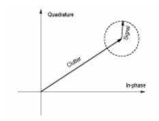
Figure M31 Phasor diagram of noncoherent MTI detector.
