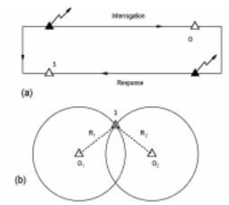
Figure N2 Range-finding navigation method.
