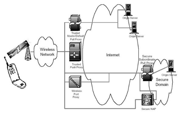
**Figure 11:** Wireless network access environment (Wireless Application Protocol, 2000). © 2000 Wireless Application Protocol Forum, Ltd. Reprinted with permission.
