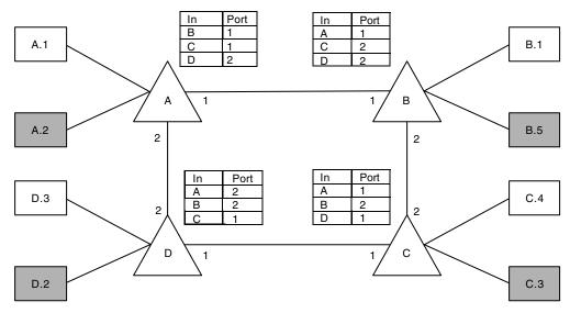
Figure 3: Example of two connectionless VPNs.
