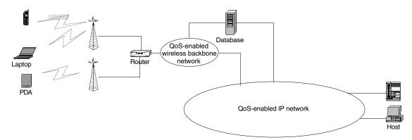
**Figure 2:** Architecture of packet-switched wireline/wireless multimedia network.
