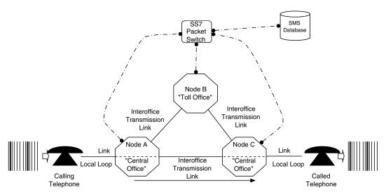
Figure 5: Conventional circuit switched telephony network.
