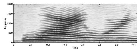
**Figure 6:** Time waveform of the utterance "Why were you away a year, Roy?" spoken by a female talker (top) and corresponding spectrogram (bottom). The spectrogram shows the power spectrum as a function of time, where the gray level indicates the power level, from low (white) to high (black).
