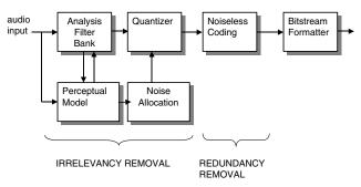
Figure 12: Block diagram of generic audio encoder.
