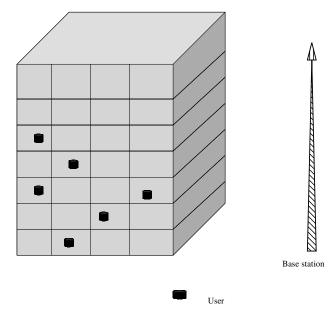
**Figure 6:** An indoor wireless system with the base station (BS) serving all the users inside. The BS may also be inside the building. The signals between the BS and the users may have to travel through several floors and partitions.
