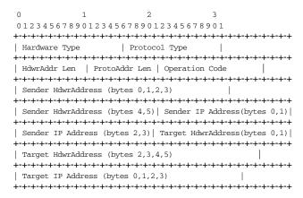
Figure 7: An ARP request/response packet.
