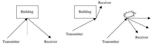
Figure 2: Various propagation mechanisms are shown: reflection (left), diffraction (center), and scattering (right).
