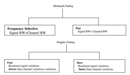
**Figure 10:** Overview of short-term fading. Pulse broadening taking place in frequency selective channel can be described in terms of the relationship between the message bandwidth and channel bandwidth. Doppler fading can be described in terms of the variations in the channel relative to the signal.
