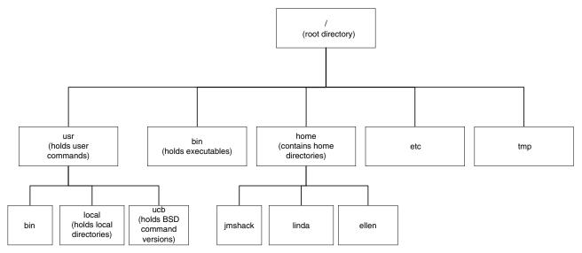
Figure 5: A typical Unix files system layout.
