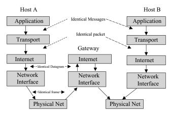
**Figure 3:** A simple TCP/IP Internet connection. Note the higher layers are not required.
