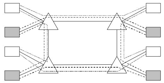
Figure 2: Example of two connection-oriented VPNs in a shared public network.
