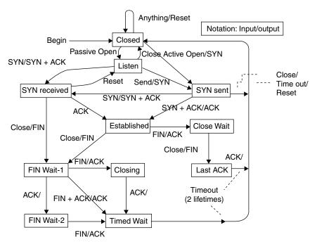
**Figure 5:** TCP state diagram.
