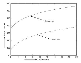
**Figure 5:** Loss predictions based on Hata model are shown. The radio frequency signal is at 900 MHz. The base station antenna height is 150 m, and the mobile unit antenna height is 1.5 m.
