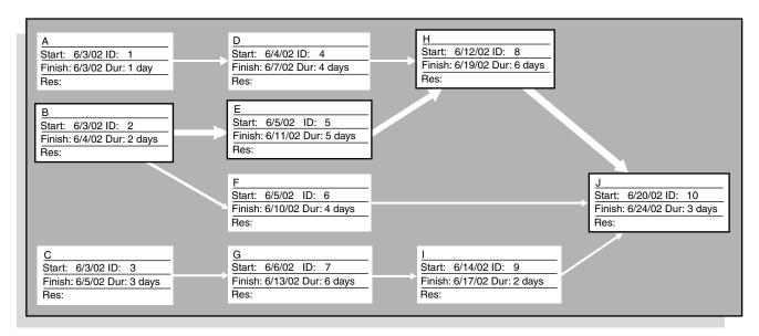
Figure 12: Network diagram and critical path in Project 2000.
