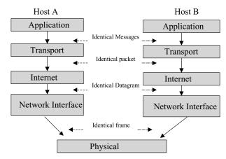
**Figure 2:** The reference model for TCP/IP. Note the lack of the session and presentation layers.
