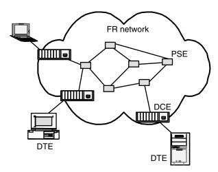
Figure 8: Frame relay network elements.
