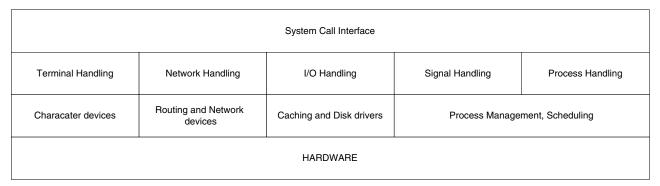
**Figure 4:** Structure of a typical Unix kernel.
