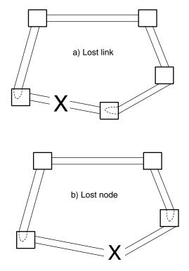
**Figure 3:** SONET ring survivability, a) lost link and b) lost node.
