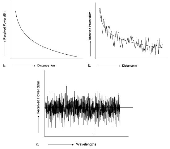
Figure 3: The plot of the received signal: (a) attenuation; (b) long-term fading; (c) short-term fading.
