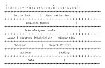
Figure 4: TCP header.
