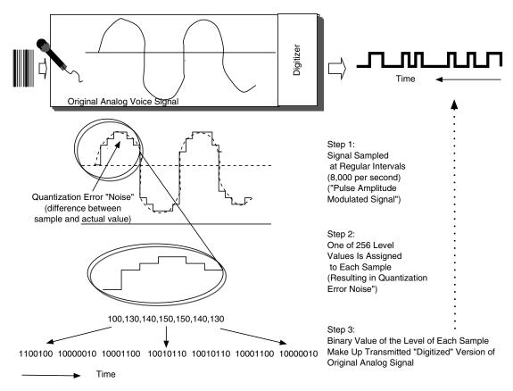
**Figure 2:** Digitization of a voice signal.
