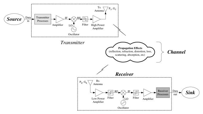
Figure 1: Simplified model of terrestrial-based RF wireless communication systems.
