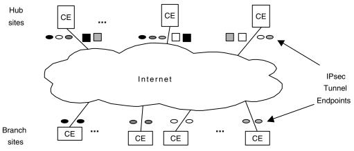
Figure 7: CE-based VPN using IPsec tunnels over the Internet.
