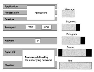
Figure 4: TCP/IP message delivery.
