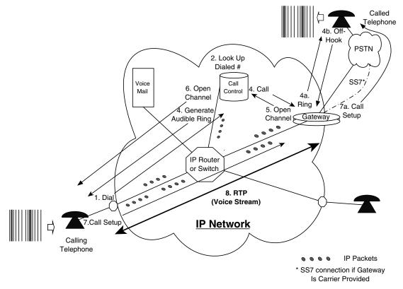
Figure 10: VOIP signaling internetworking with public switched network (PSTN).
