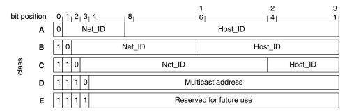
**Figure 12:** IPv4 addressing format.
