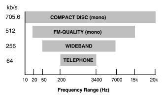
Figure 1: Relationship between bandwidth and bit rate.
