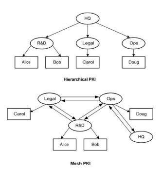
**Figure 3:** Hierarchical PKI and mesh PKI architectures.
