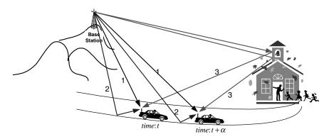
Figure 6: Interference of radio wave.
