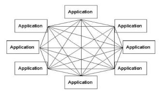
**Figure 4:** Point to point-integration structure.
