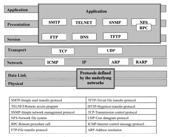
Figure 3: The OSI model and the TCP/IP protocol.
