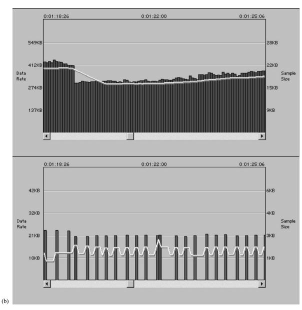
**Figure 1:** (a) Images of frames numbered 1231–1233 from the NASA budget FY 2001 movie "The Emotion of Space" showing scene change at frame 1232 and motion sequence from frames 1232 to 1233. (b) Graph showing data rate and sample size by frame centered at time code 0:01:22:00 (frame 1231) for H.263 compression of the above movie at 15 fps and average data rate 293 and 14 kbps, respectively.
