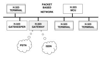
**Figure 15:** An example network topology using the H.323 protocol.
