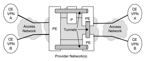
Figure 5: Generic PE-based (also called network based) VPN.
