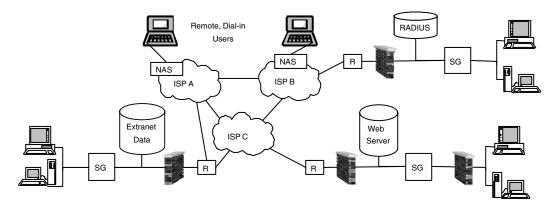
Figure 8: Pure IP-distributed VPN design.
