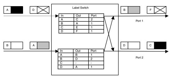
Figure 1: Illustration of layer 2 label switching.
