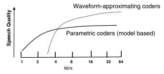
**Figure 5:** Quality vs. bit rate curves for waveform and parametric coders.
