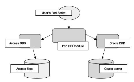
**Figure 1:** DBI provides an abstract interface for specific database systems.
