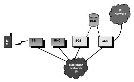
**Figure 4:** Architecture of a UMTS network.
