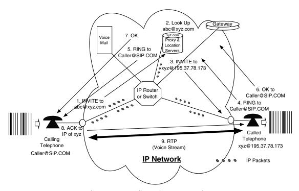
Figure 9: VOIP call routed using SIP signaling.
