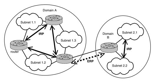
Figure 11: Routing within and between autonomous domains.
