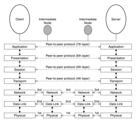
Figure 2: Messaging delivery using OSI model.
