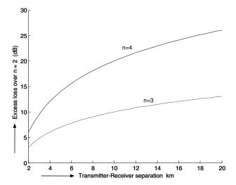
**Figure 4:** The losses at n = 3 and n = 4 are compared with the free space loss (n = 2).
