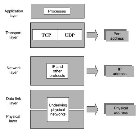
**Figure 5:** Address types and assignments in TCP/IP protocol.
