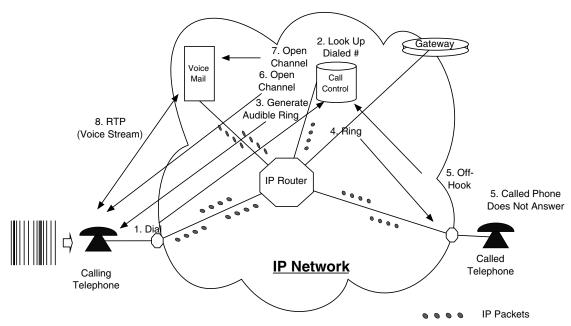
Figure 8: Called telephone unavailable with reroute to voice mail with H.323-type signaling.
