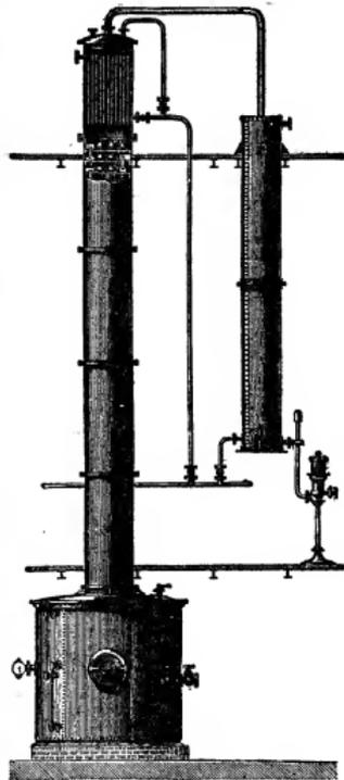
FIG. 4.—Benzol Still (elevation).
