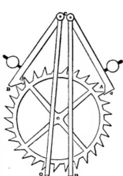
FIG. 17.—Mudge's Gravity Escapement.
