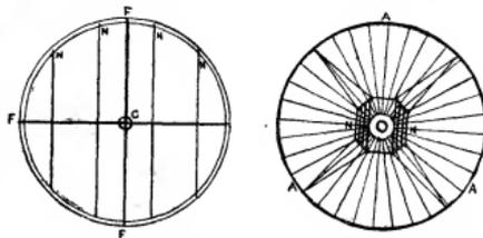
Fig. 2.—Admiralty Compass (Frame and Needles). Fig. 3.—Thomson's (Lord Kelvin's) Compass (Frame and Needles).
