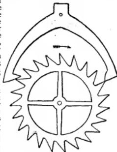
FIG. 8.—Anchor or Recoil Escapement.
