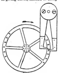
FIG. 10.—Pin-Wheel Escapement.
