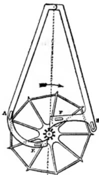
FIG. 18.—Bloxam's Gravity Escapement.
