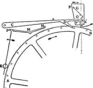
FIG. 21.—Chronometer Spring Remontoire.
