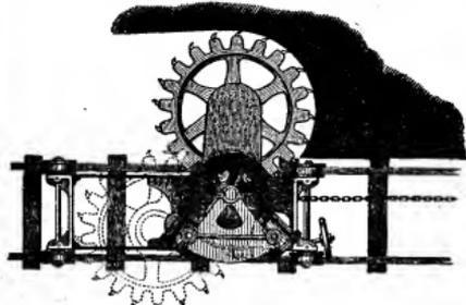
FIG. 11.—Winstanly & Barker's Coal-cutting Machine—Plan.
