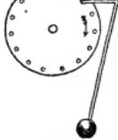
FIG. 2.—Galileo's Escapement.
