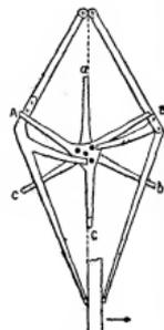
FIG. 20.—Double Three-legged Escapement.
