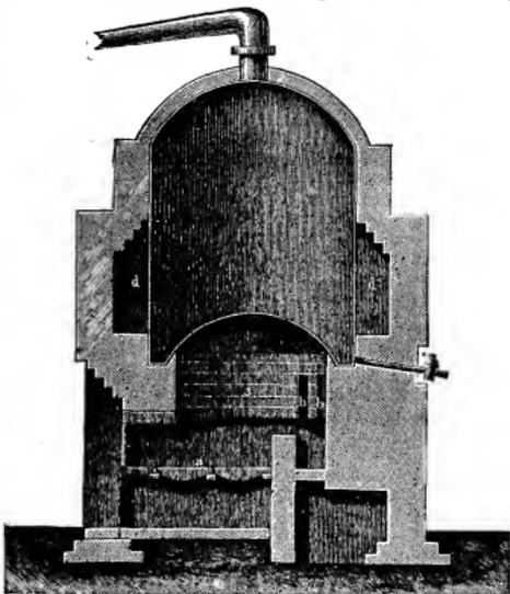
FIG. 1.—Tar-Still (sectional elevation).<sup>1</sup>
