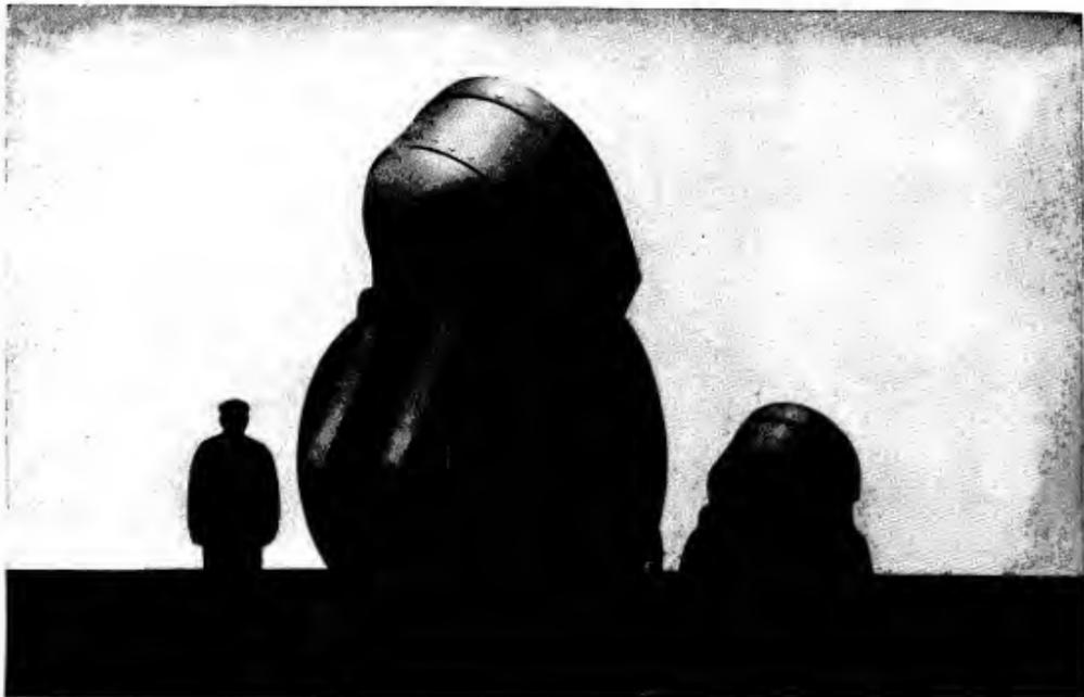
FIG. 11.—BUCKETS OF 5 AND 54 CUBIC FEET CAPACITY COMPARED.
