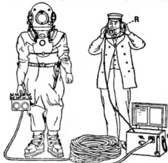
FIG. 4.—Diver's Telephone Communication with the Surface.
